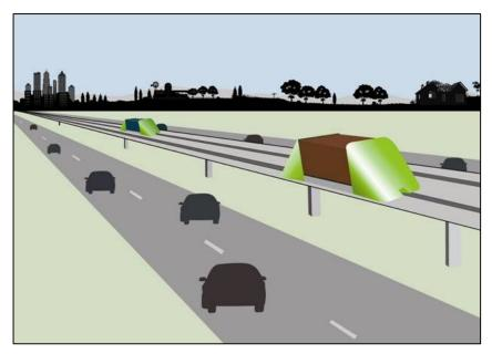
The diagram illustrates what the freight shuttle could look like: an elevated, unmanned track with single load transporters going in both directions. At destination, the transporters would enter cargo bays terminals at which point the trailers would simply hook up with a traditional big rig to get a short distance to a particular store.
